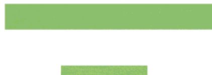
FIG. 3. An area of colored paper that, illuminated by daylight, with its white surround, well approximates the appearance, to one or other of the CIE Standard Observers, of objects 2 and 1 of Fig. 2. That is, to a normal human observer, the lights reflected in daylight by objects 2 and 1 are an acceptable white-light match, while to either CIE Standard Observer, they appear as strong green and white, respectively.
