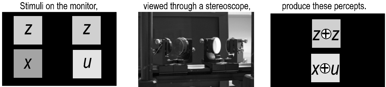
Figure 1: Stimulus in brightness matching task: from what is displayed on the monitor to what respondents see. The x, u, z are luminance values. The task: respondents adjust the luminance z until they are satisfied that z \oplus z is equivalent to x \oplus u in brightness.
